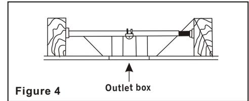
To hang your fan where there is an existing fixture but no ceiling joist, you may need an installation hanger bar.(Fig.4) (available at any Home Depot store).
