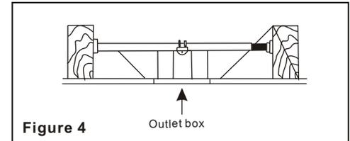
To hang your fan where there is an existing fixture but no ceiling joist, you may need an installation hanger bar as shown in Figure 4 (available at your Hampton Bay Retailer).
