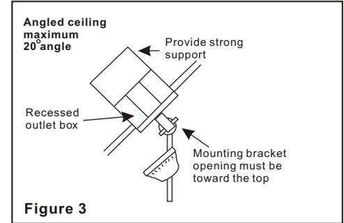
Note: You may need a longer downrod to maintain proper blade clearance when installing on a steep, sloped ceiling.
